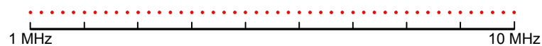
Fig. 6-13: Linear x-axis scaling: the distance between the sweep points is equal, e.g. 200 kHz
