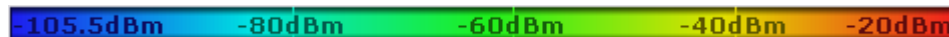
Fig. 7-9: Linear color curve shape = 0; colors are distributed evenly over the complete result range
